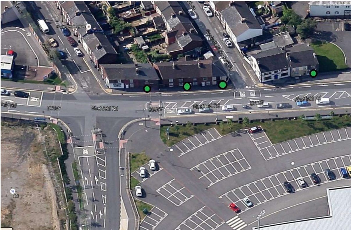
Figure 4: Locations of Diffusion Tube monitoring on the affected façade
