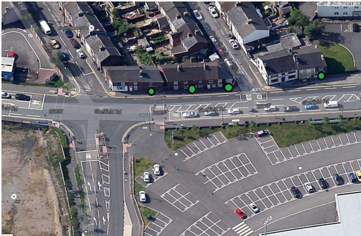
Figure 4: Locations of Diffusion Tube monitoring on the affected façade
